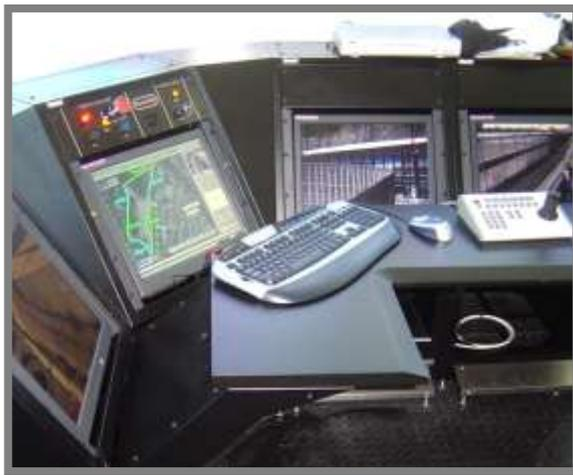
The PC monitor displays the present status of the entire perimeter in real time. The main screen displays a color graphic map of the secured site, clearly showing the perimeter zones in different colors. When an alarm is triggered the relevant zone will start blinking in red and an audible alarm will sound. From the main screen, the operator may use different keys to move through the system's functions such as:
